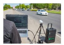
The video camera is mounted on the side of the road to capture the passing cars. The signal from the camera is transmitted to the laptop with the pre-installed Road Bailiff software and regional debtor databases. The software recognizes number plates of passing vehicles and checks them against the current databases. is found in the database, the image of the debtor's vehicle is displayed on the laptop screen, and a sound signal is given.
